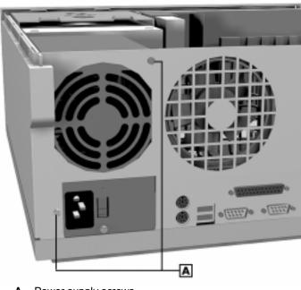
Removing the Power Supply Screws
